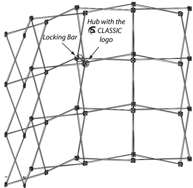
**IMPORTANT NOTICE:** The locking bar is for set-up only. It MUST be RELEASED before hanging the panels. If the panels do not fit, then the locking bar has not been RELEASED.
